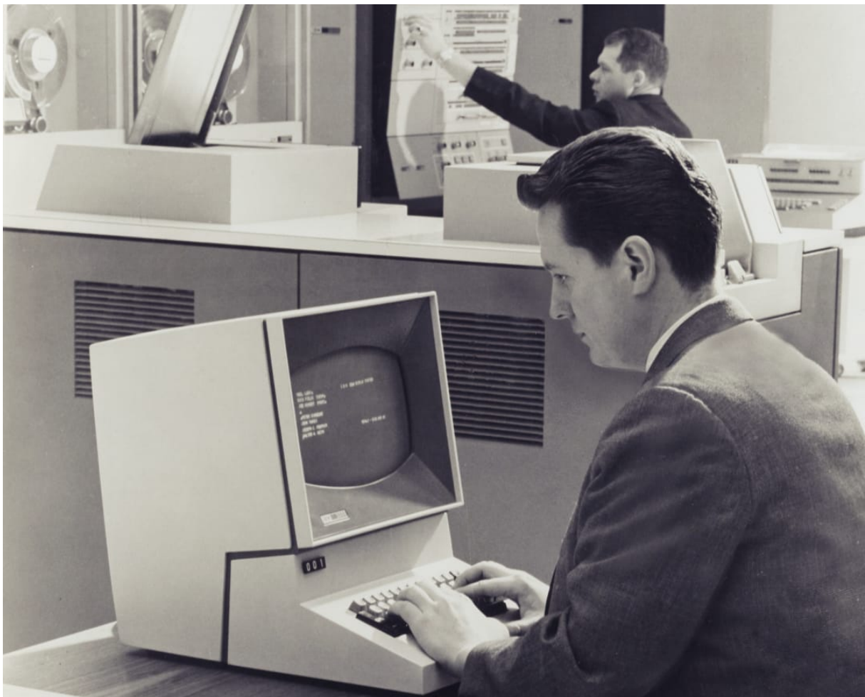
Figure 1.1: The IBM 2260 display-based terminal. Credit: Norsk Teknisk Museum.
